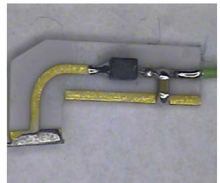
Surface Mount Components on a Ceramic Blade Probe
