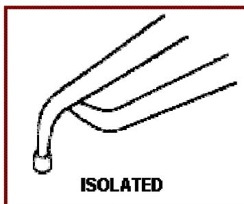
The isolated edge sensor is an SPST NC switch, which is electrically isolated from the device surface by a jewel bead.
