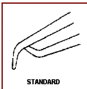
The standard edge sensor application is a simple SPST normally closed (NC) switch consisting of a probe and a switch portion. The probe needle (sometimes called a contact) is permitted to touch the device surface and if forced upward allowing separation from the switch.
