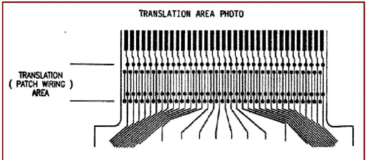
The principle objective of a probe card is to properly connect a test pad to a probe through the printed circuit traces to the edge connector, which interfaces with the tester. A particular test pad ultimately connects to one port of the tester, which is sometimes referred to as a scanner.
